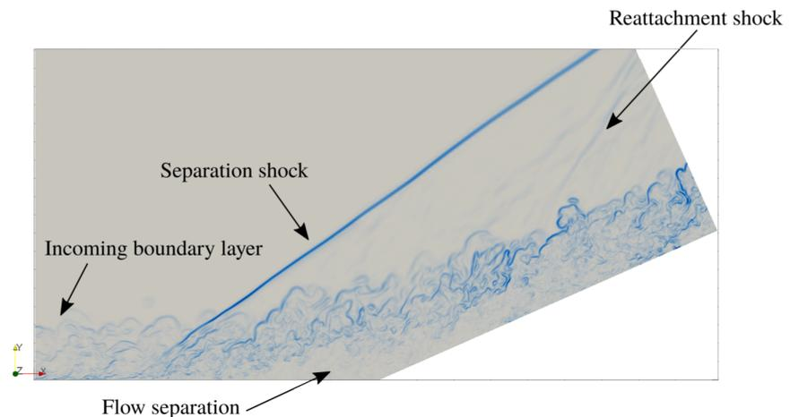
Figure 1: Numerical schlieren of the shock-wave / boundary layer interaction in a compression ramp flow
