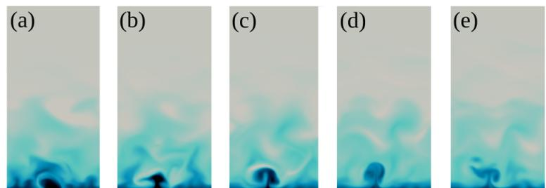
Figure 2: Flow field in the vicinity of the air-jet vortex generator. Sub-figure (a) is at the location of jet injection, (b-e) are the downstream locations.
