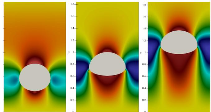
*Rising bubble undergoing deformation.*
